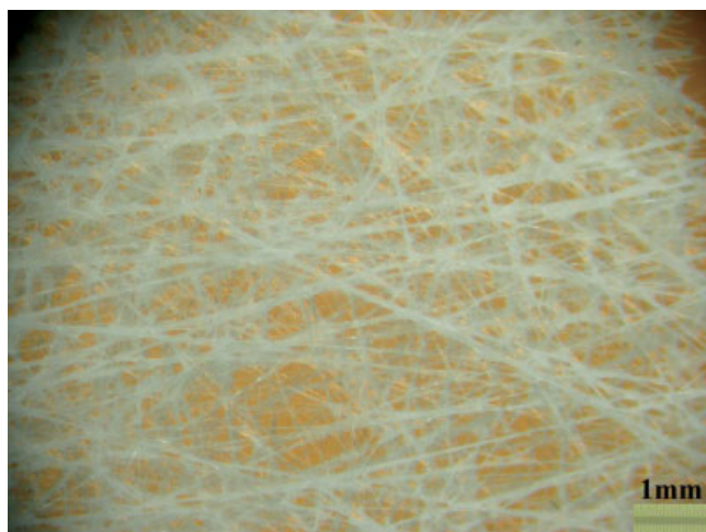
Figure 1 Morphology of the glass fiber. [Color figure can be viewed in the online issue, which is available at www.interscience.wiley.com .]
